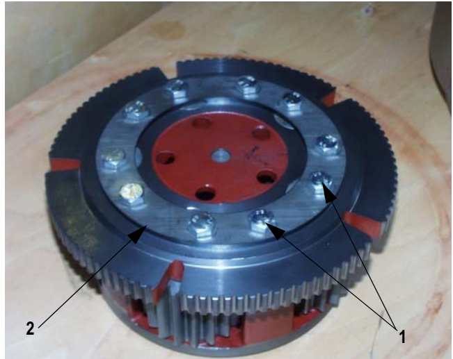
Picture 4 Planetary gear removed
