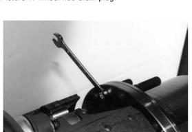
Picture 2. Unscrewing hub housing retaining screws.
