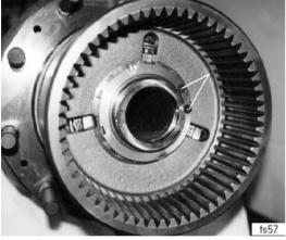
9. Remove the ring gear and the ring gear hub from the axle tube (Picture 8.). The outer bearing will follow the ring gear hub. To make removal easier, support the wheel hub.
