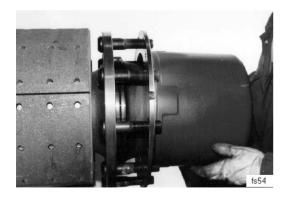
Picture 3. Hub housing removal.
