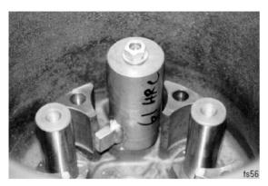
Picture 6. Planet gear shafts removing with a special tool.
