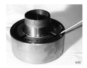
Picture 9. Retaining ring removal.
