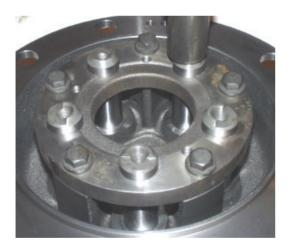
Picture 13.Installation of the planet gear shafts.
