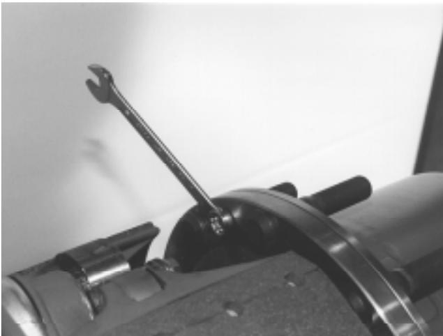
**Picture 2.** Unscrewing hub housing retaining screws.
