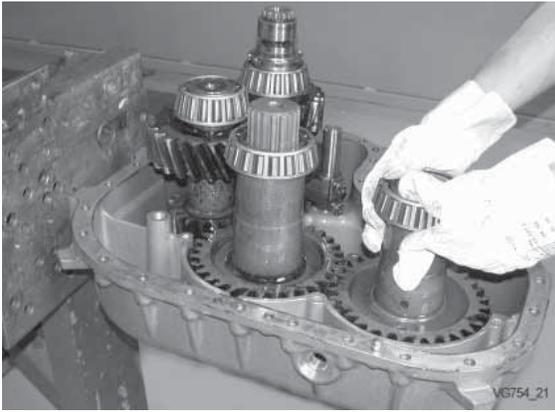
Lift out intermediate shafts and output shaft.
