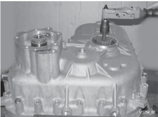
Check the rolling torque of the rear axle output shaft.
