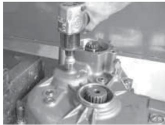
Disassemble oil tube.
