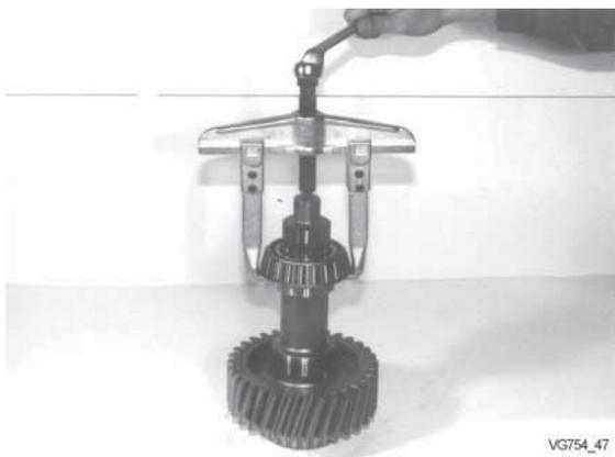
Pull off the rear tapered roller bearing.
