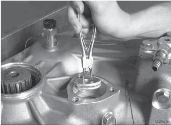
Pull off piston with sealing.
