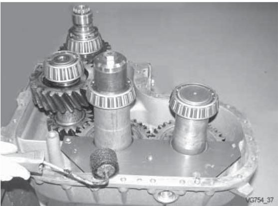
Apply **LOCTITE 518** on front housing.
