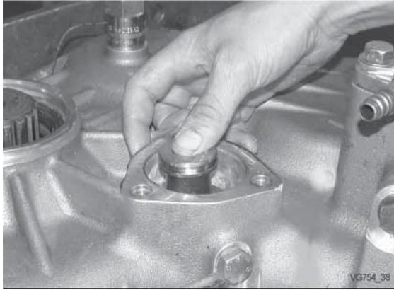
Slide cylinder and seal on shift rod.
