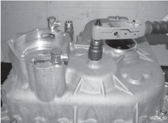
Check rolling torque of the double gear.
