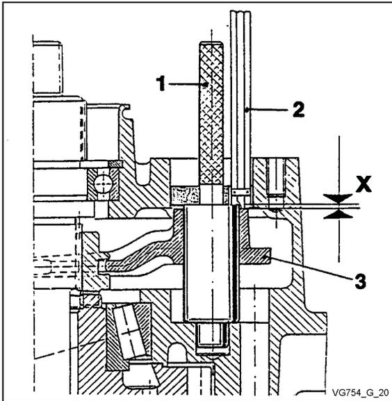
Measure distance **X** between assembly tube (pos. 1) and shift fork (pos. 3).
