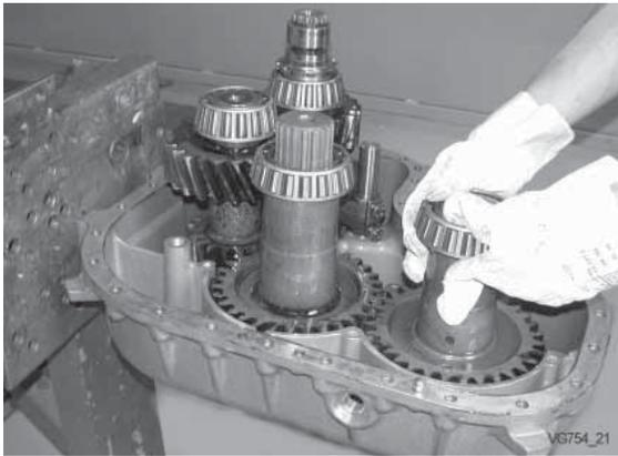
Install intermediate shafts and output shaft.
