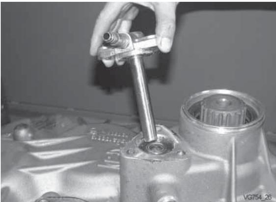
Remove cover and shifting shaft together.
