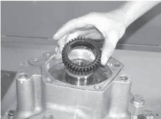
Remove oil pump gear.
