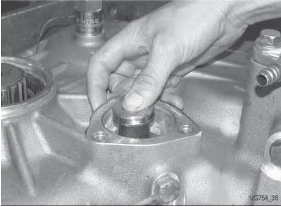
Slide cylinder and seal on shift rod.
