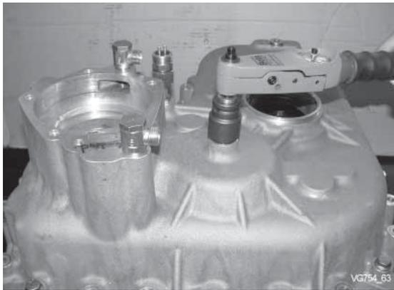
Check rolling torque of the double gear.
