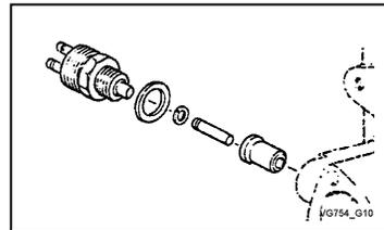
Mount sliding bush, pin and monitor switch
