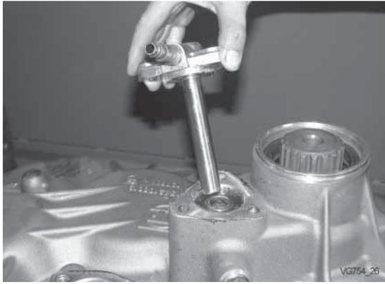
Pre-assemble cover and mount together with selector shaft into shift cylinder.
