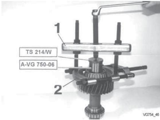
**1.7 Dismantle rear axle output shaft:**
