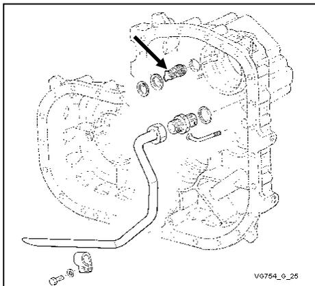
Mount suction line with fitting and spray tube.
