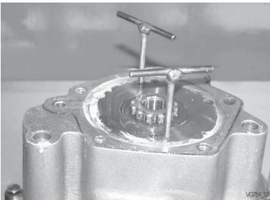
Lift off oil pump housing.
