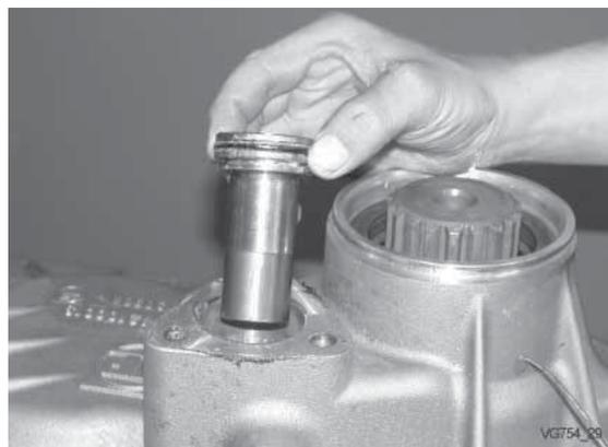
Install shifting piston with seal.
