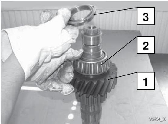
Mount gear (pos. 1) on shaft.
