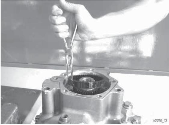
Remove outer oil pump gear.
