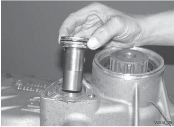
Remove shifting piston with seal.
