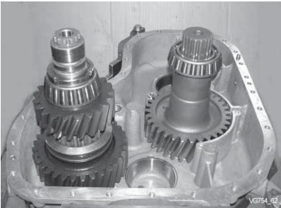
Setting of rear axle output shaft and input shaft:
