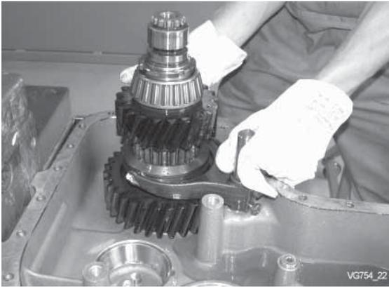
Lift out input shaft together with shifting.
