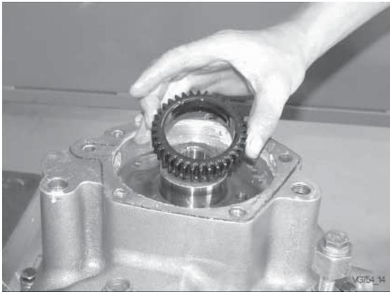
Install oil pump gear on input shaft.
