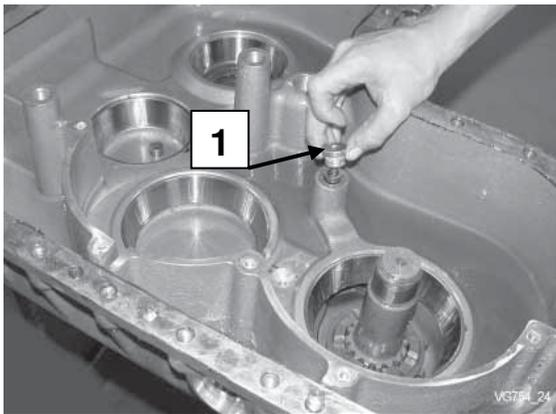
Slide in shaft spring (1) and plug.
