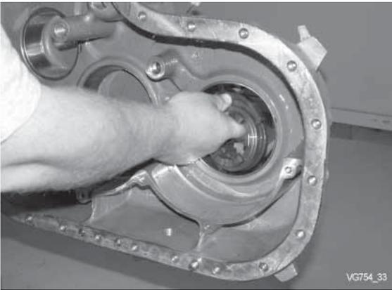
Remove shifting fork and shifting dog sleeve.
