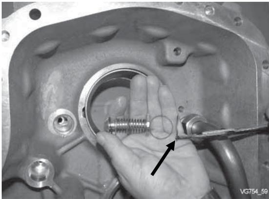
Secure bypass valve with retaining ring.
