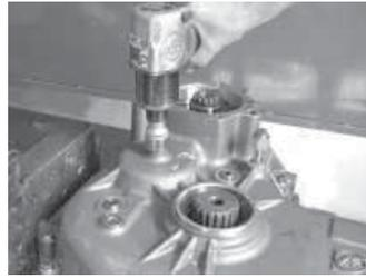
Disassemble oil tube.
