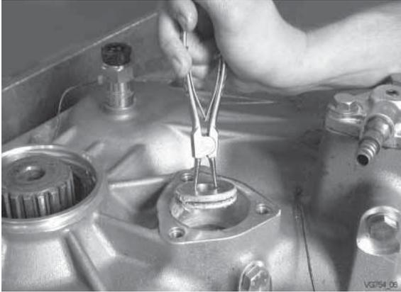
Pull off piston with sealing.
