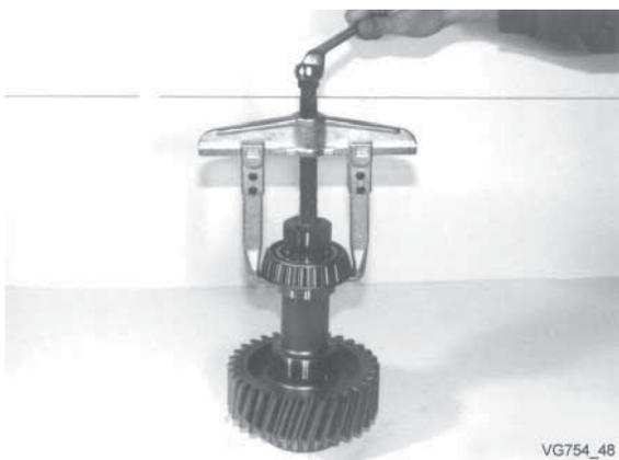
Pull off the rear tapered roller bearing.
