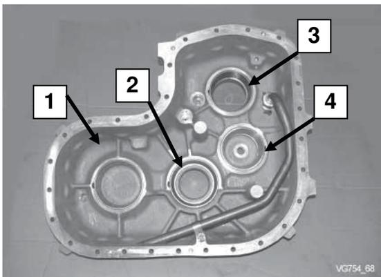
Mount bearing outer rings into the housing cover.
