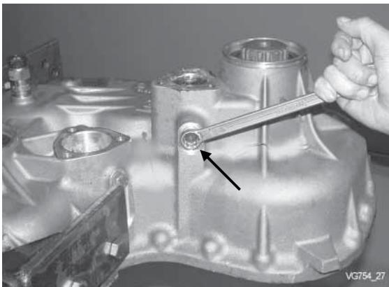
Install sliding sleeve, plug and control switch.
