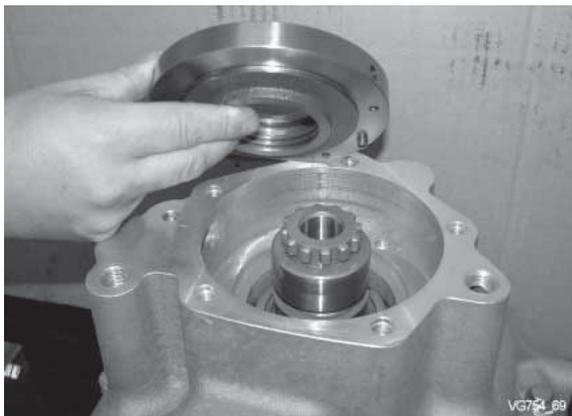
Disassemble oil pump cover.
