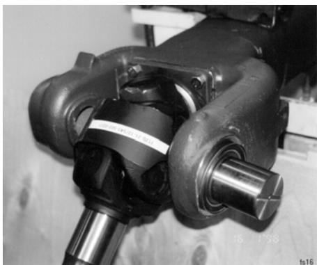
Picture 25 Axle housing end with the lower king pin with the gamma seal as well the drive shaft.
