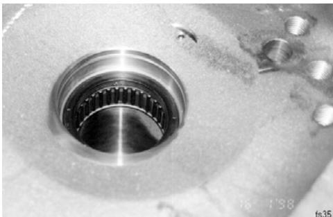
Picture 44 Needle bearing ready installed.
