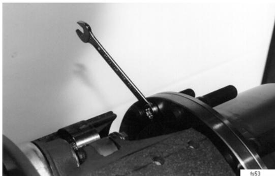
Picture 6 Unscrewing hub housing retaining screws.
