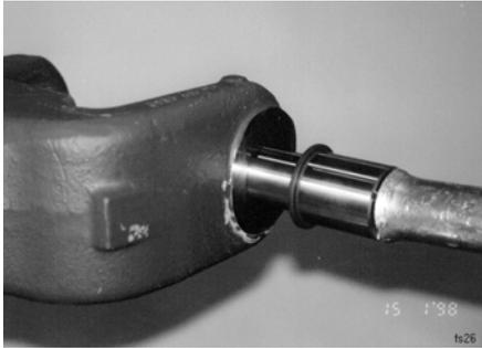
Picture 35 Installation of the lower king pin.
