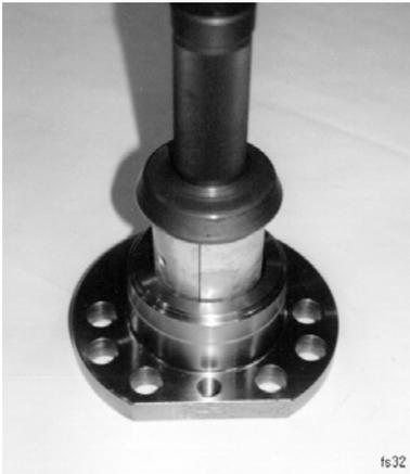
Picture 41 Lower king pin bearing bush being installed into the flange bore.
