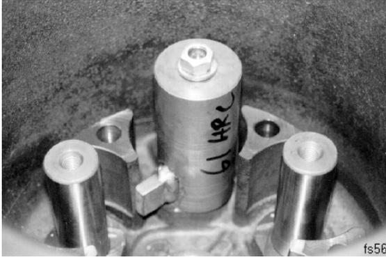
Picture 10 Planet gear shafts removing with a special tool.
