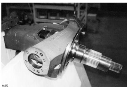
Picture 24 Steering knuckle ready to be removed.
