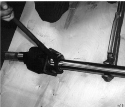
Picture 28 Opening of the drive shaft support bearing nut
