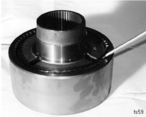
Remove the retaining ring. Remove the ring gear from the ring gear hub by tapping lightly with a soft metal hammer.
