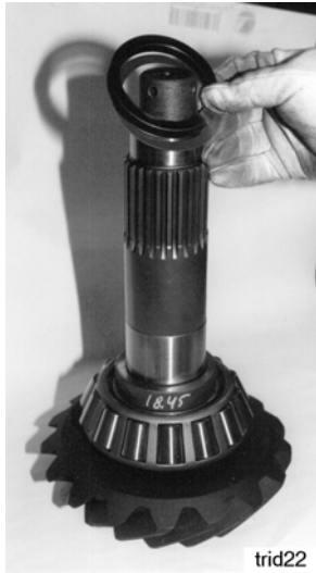
Picture 12: Pinion with inner bearing installed
