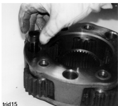
Picture 25: Installation of planetary carrier cover screws.
