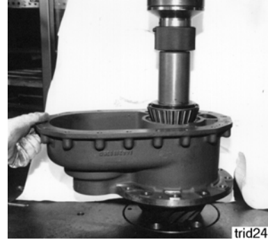
Picture 13: Pinion bearing installation and adjustment
