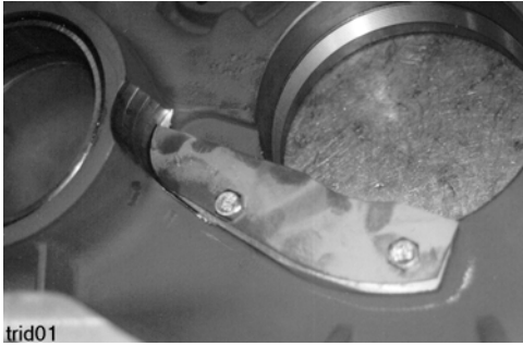
Picture 32: Oil retaining plate in the housing
