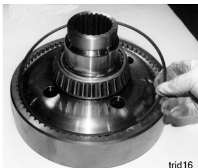
Picture 21: Installation of the ring gear hub locking ring.
