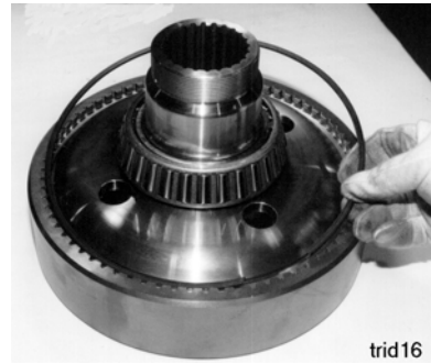
Picture 9: Removal of the planetary hub locking ring
