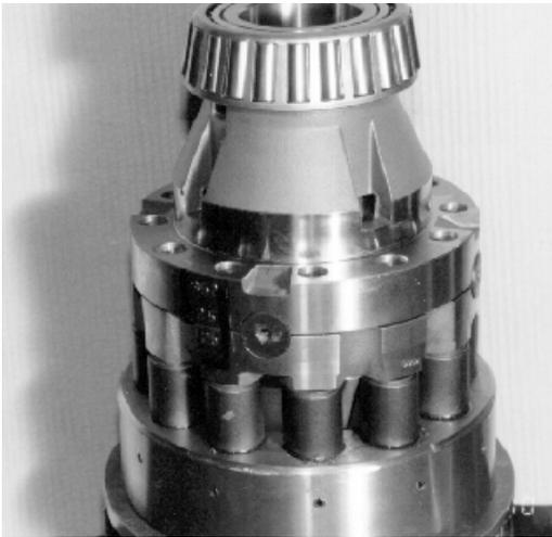
Picture 18 Assembled differential without the crown wheel
