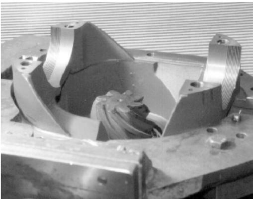
Picture 19 Drive gear housing ready for installation of the differential assembly
