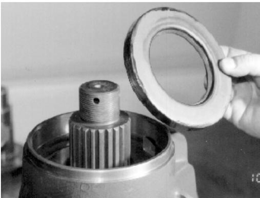
Picture 13 Pinion seal ready for installation.
