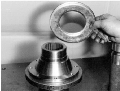
Picture 14 Seal protection plate ready for installation.
