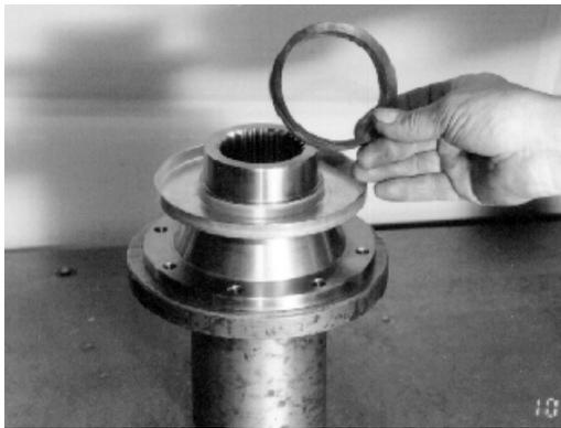
Picture 15 Seal protection plate installed onto the flange. V-seal ready for installation.
