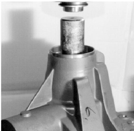
Picture 8 Removal of pinion in workshop press
