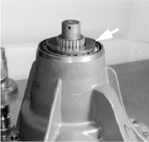
Picture 11 Pinion installed in the housing. Press on the inner race on the spot indicated by an arrow by a suitable drift first until it stops and then for testing of adjustment by a force of 16 ton.
