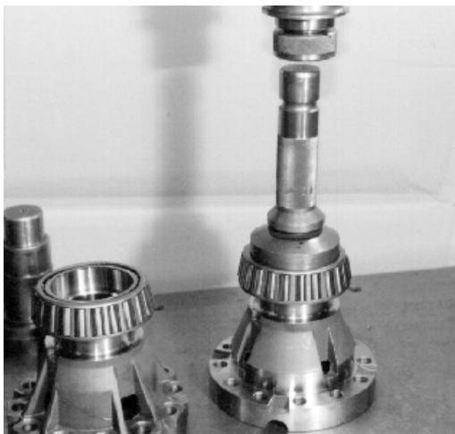
Picture 16 Pressing of a conical roller bearing to a differential casing half.
