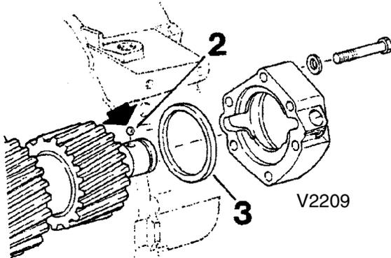
Set driving ball (76/2) into bore of intern. shaft.
