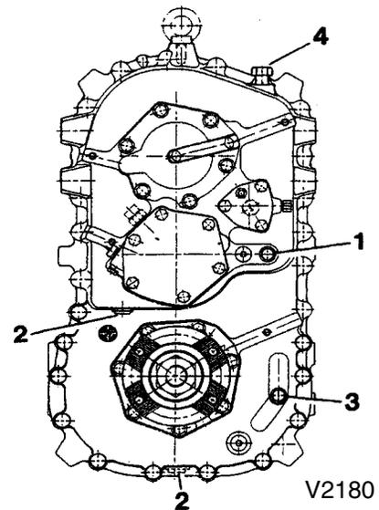
Drain oil by unscrewing both oil drain plugs (2)
